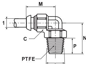
Threads are treated with PTFE sealing material
