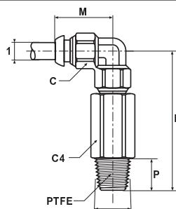
Threads are treated with PTFE sealing material
